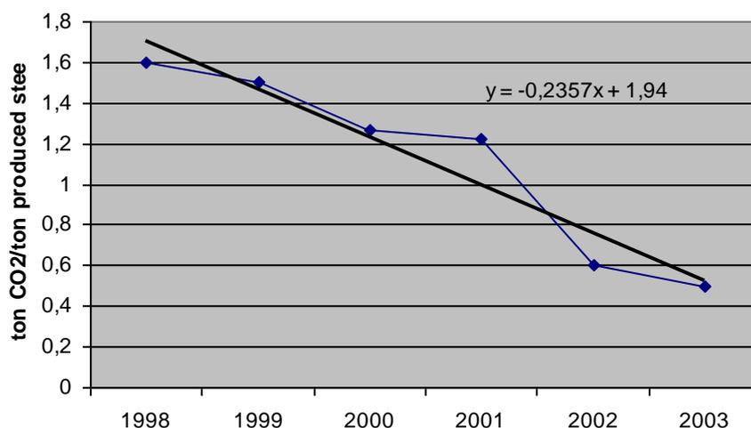
**Figure 2.1** Example (Not Outokumpu) of a diagram with the quota ton CO<sub>2</sub> emitted from input materials per ton produced steel and a resulting trend line
